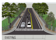
Standard collector-arterial intersections may be retrofitted with Bicycle Lanes and Bicycle Boxes. Bicycle Boxes may also be equipped with Signal Detection equipment and other countermeasures, such as peg-a-tracking. Cities like Portland have discovered that Bicycle Boxes can be enhanced by the use of colored pavement.
